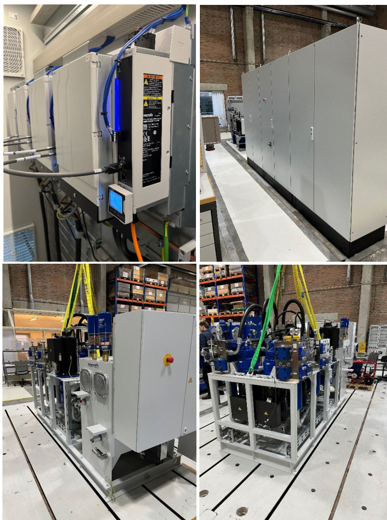
Fig. 4.2. eCHASPOR prototype about to be installed a laboratory at Aalborg University.
