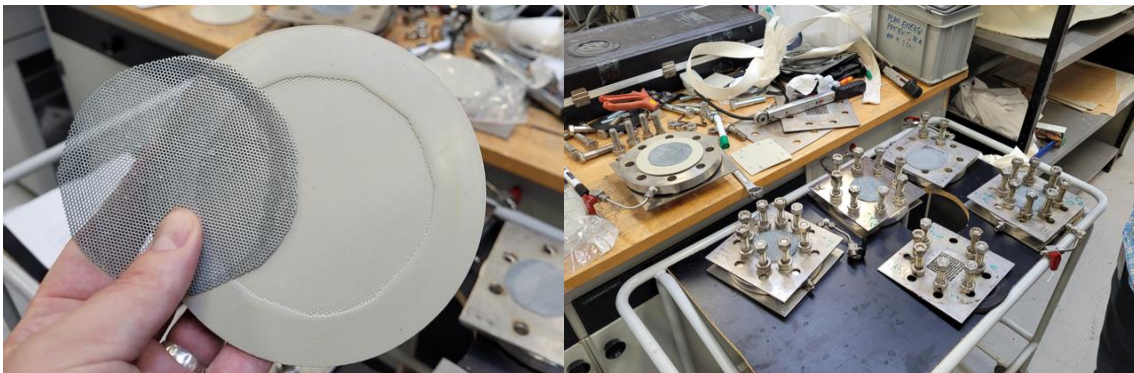
Figure 6. Sample Preparation at DTI (a fine mesh is used to expose the liner to pressurized water on one side and air on the other side)
