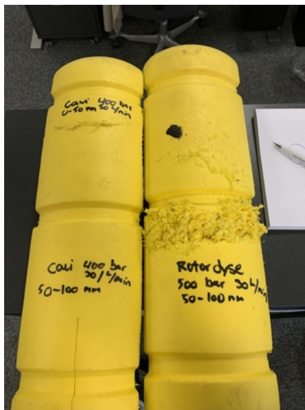
Figure 12 Cavitation technology to the left. Water jet to the right. Shows that cavitation technology is more gentle to surface material.
