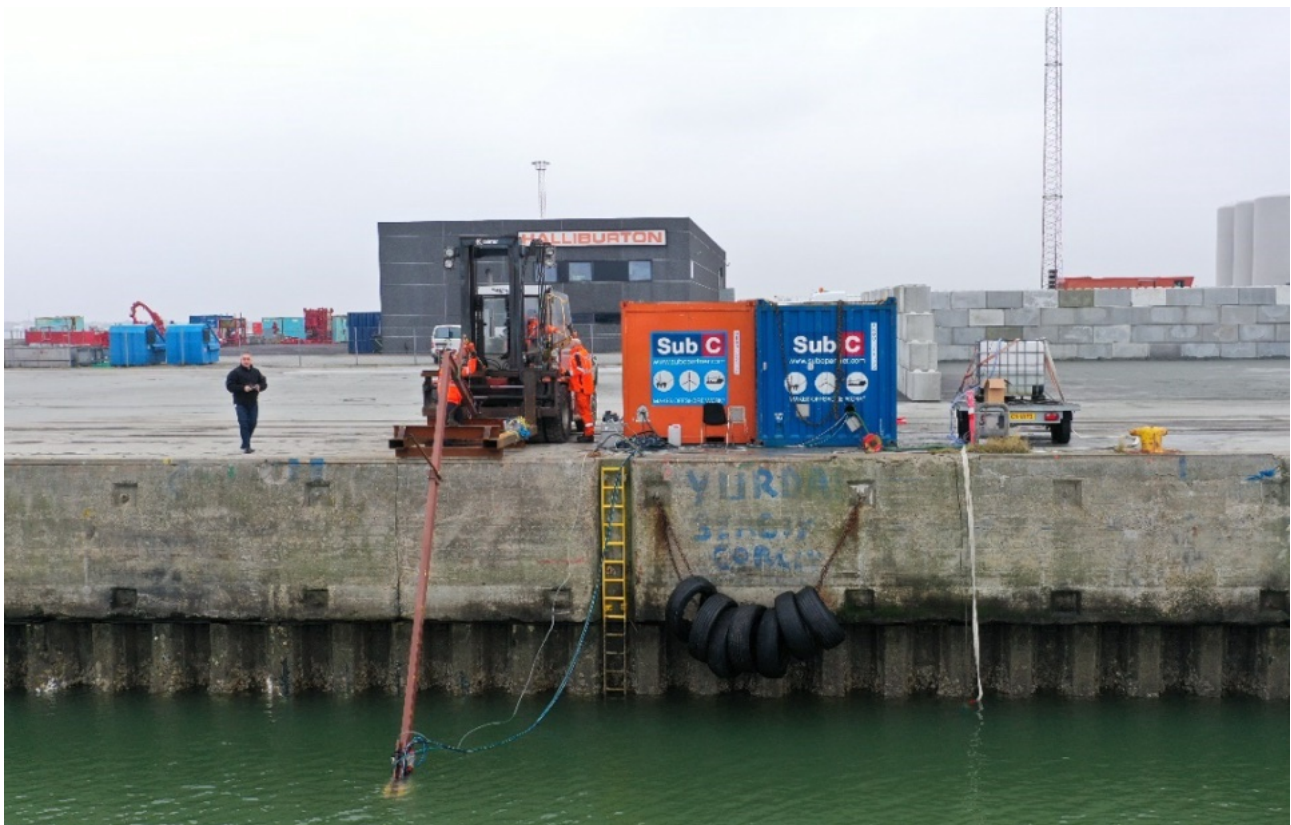
Figure 9 Test setup with tool container, control container and structure to carry the cleaning tool.
