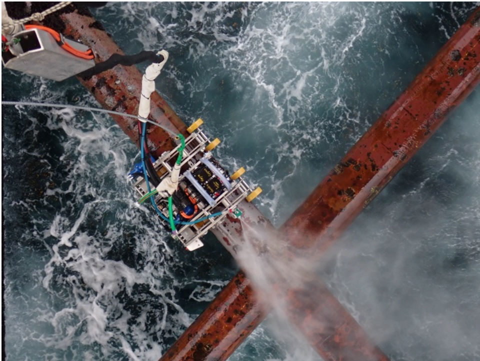
Figure 4 Example of solution fixes to the structure (Robotic Crawler by SubC Partner)
