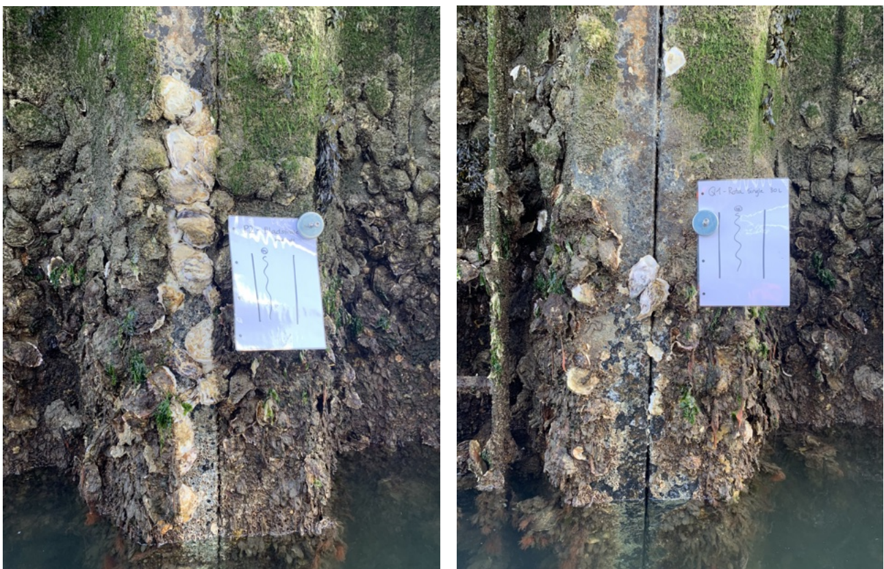
Figure 10 Poor performing water jet nozzle (left) vs. well performing water jet nozzle (right) after one run.
