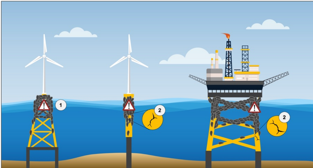
Figure 1 Due to additional loads and accessibility for inspection, it is important to remove MG.
