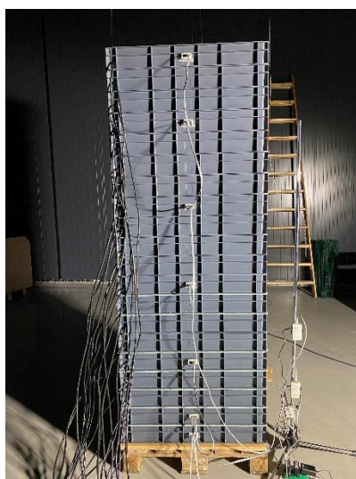
Figure 2: 20 stacked customized production trays with heating elements and temperature measurements.
