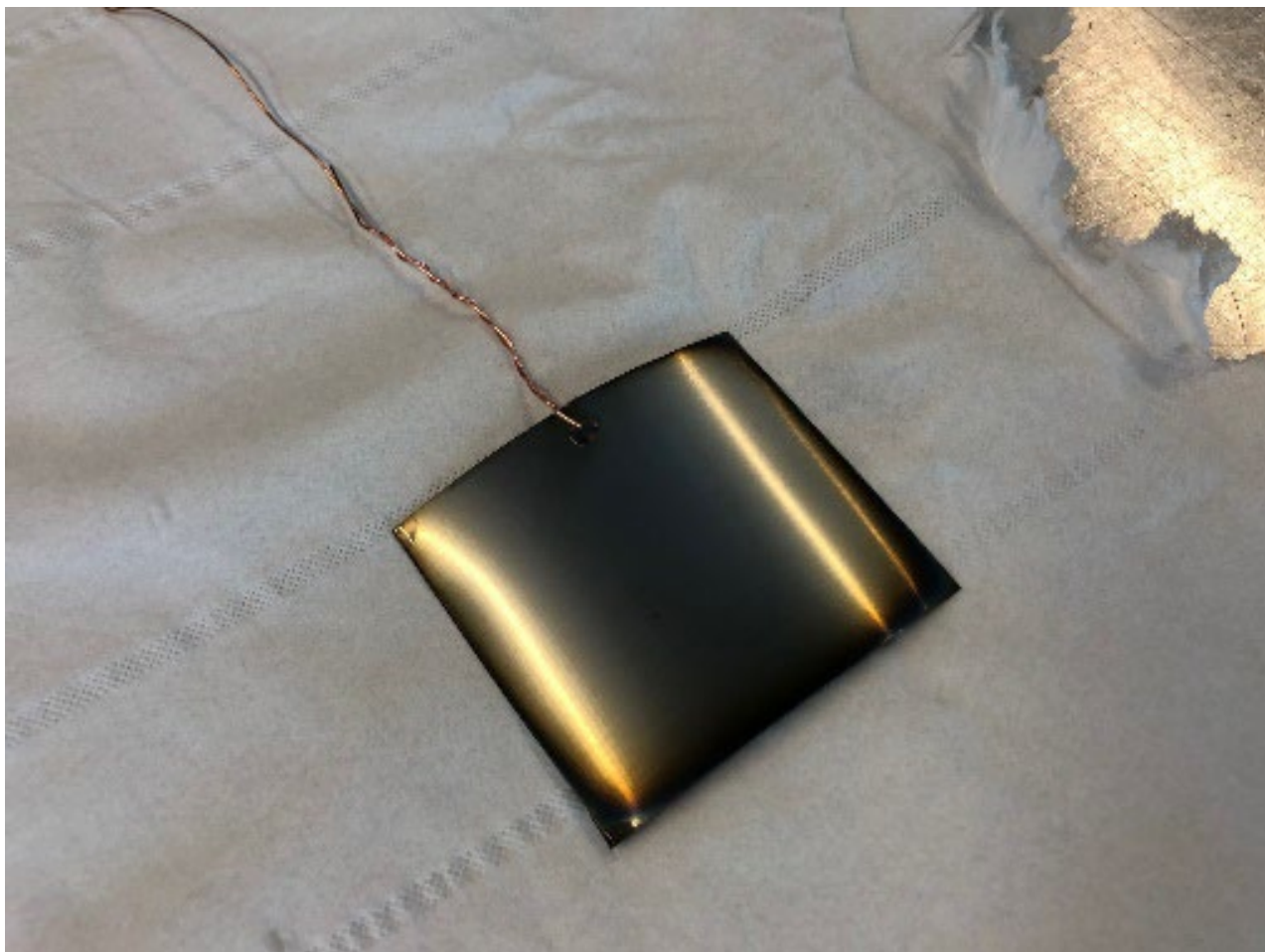
Figure 9: Photo of molybdenum sheet after anodizing treatment
