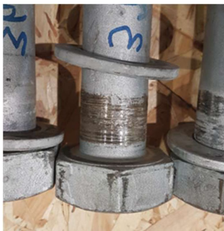
Figure 10: (left) wear damage of the zinc coating on the bolt shank underneath the head due to head-torque and (right) in the bolt garniture assembly shown any water present in the flanges during installation is trapped and can lead to ice formation in sub-zero site conditions.
