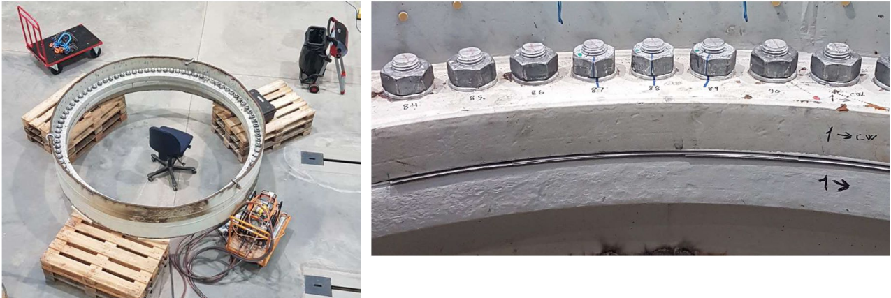
Figure 9: (left) Off-cut of a NM 52-900 tower ring flange setup at the Large-Scale Testing Facility at DTU Wind and (right) detail of the ring flange bolts (bolt nuts facing upwards) with a shim placed in-between the flanges to simulate the effects of a flange gap.
