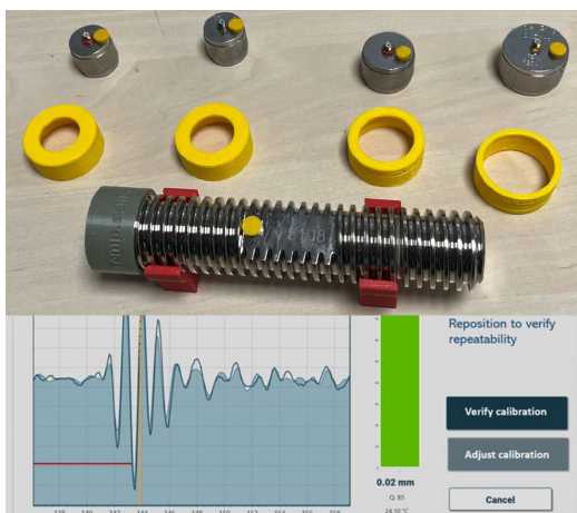
Figure 8: (left) Center pads (yellow rings) and different corresponding sensor types and (right) elongation error of measurements as a function of temperature and bolt length.
