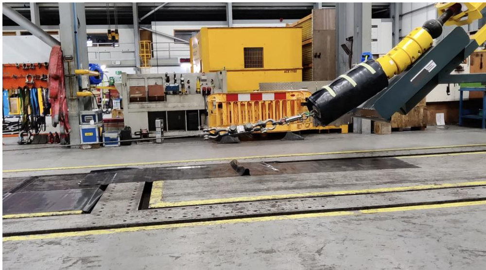
Caption: Weak link breaking and cable recoil test during Yard Trial 2024
