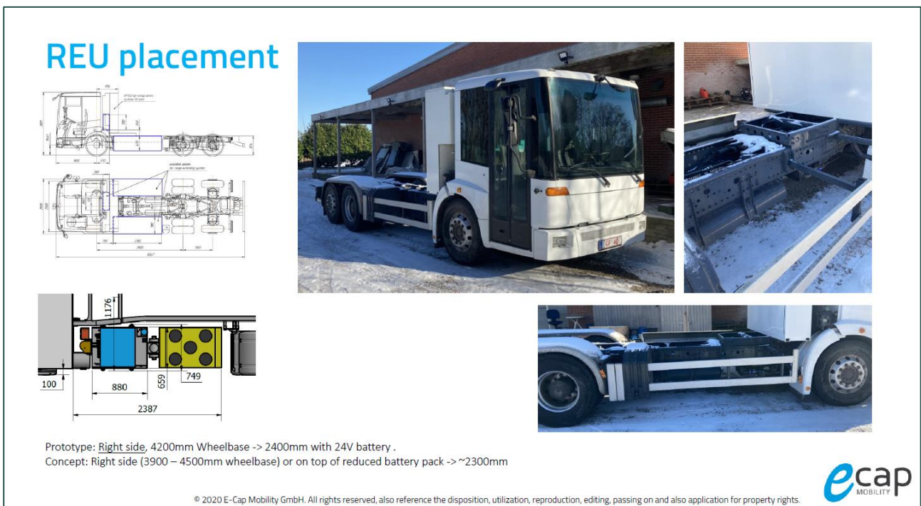
Figure 1: Proposed location of 63kW fuel-cell stack
