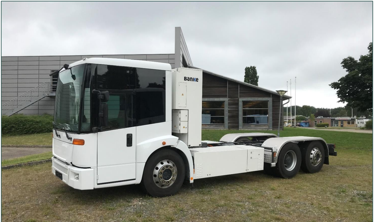
Figure 4: Side view of converted truck with hydrogen tank between axles
