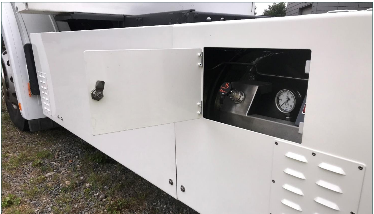
Figure 5: Close up of hydrogen tank and fuelling nozzle
