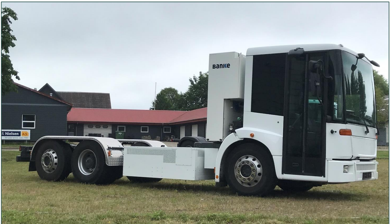
Figure 3: Side view of converted truck with fuel-cell stack between axles
