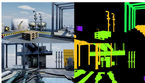
Figure 3 - Examples of images generated with Isaac Sim (left) with associated object segmentation masks (right).
