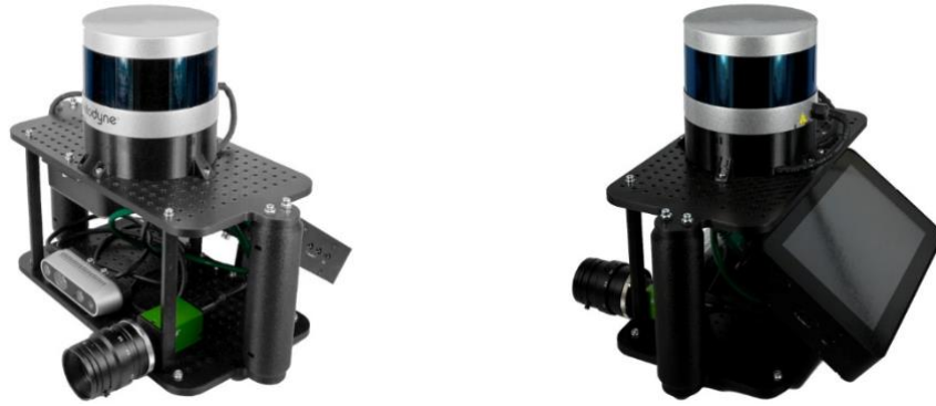
Figure 7 - Front and back views of the Mobile Data Recorder. The device integrates a LiDAR sensor, camera, and single board computer into a handheld unit. It features a built-in touchscreen interface with an integrated capture button, allowing users to preview and record images during inspection.
