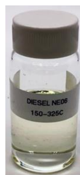
Figure 5. Diesel derived from digestate fibers
