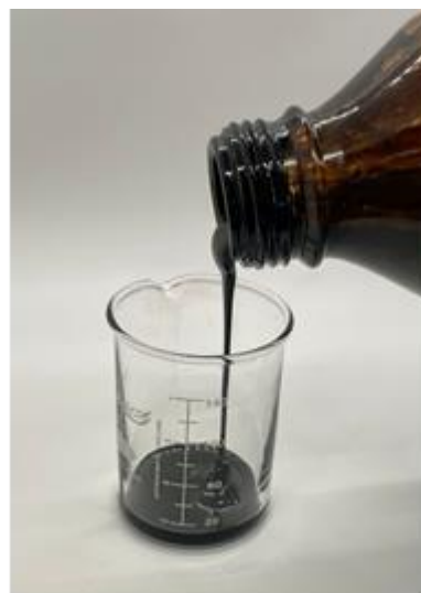
Figure 3. Digestate-fibers derived HTL biocrude at 25°C
