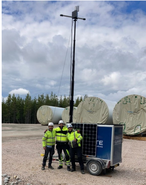
Solar trailer with mast extended. Picture is from the first pilot project (Björnberget). Cameras can be seen at top of the mast.
