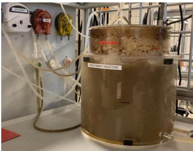
Figure 3: Sequencing batch bioreactor used for investigating the aerobic treatment of HTL process water.
