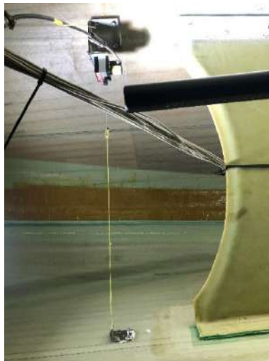
Figure 29. Wire potentiometer measuring relative out-of-plane deformation of the pressure side trailing edge panel
