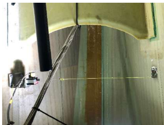
Figure 43. The mounted wire potentiometer measured out-of-plane deformation of the blade panels. The potentiometer was installed 3.8m from the root and 200mm from the retrofitted aft shear web.
