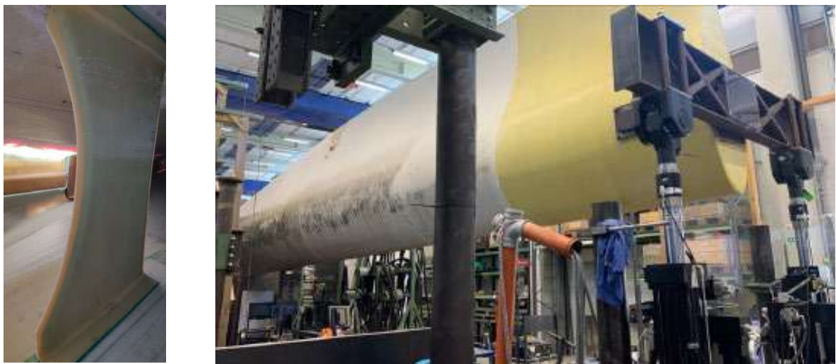
Figure 13: The installed artificial aft shear web (on the left), the SSP34m blade cut-out installed on the test rig at DTU Construct's Structural Lab (on the right)
