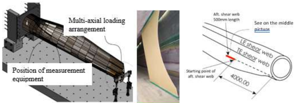
Figure 40. Large-scale strong-floor based test setup, the root section is mounted on a vertical strong-floor and the tip end is mounted onto the load train, the load introduction is explained on Figure 6 (left). Retrofitted aft shear installed in the 2 blade cut-outs (middle). The position of the retrofitted aft shear web illustrated (right).
