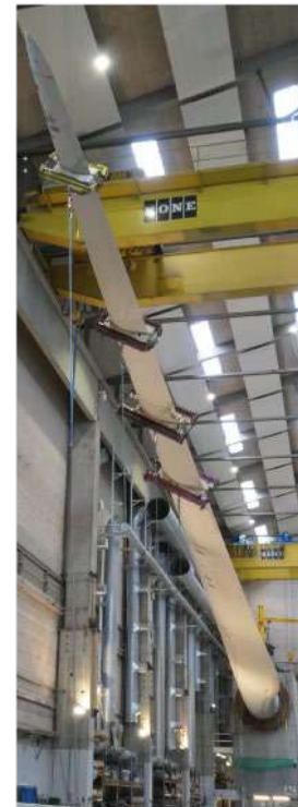
Figure 51: Sketch of a full-scale static test setup with applied torsional load components (left). Photo to the right show a full-scale test of a LM58,7m blade with combined static loads performed at a commercial test center in collaboration with LM-Windpower and Bladena, see ref. [1] EUDP RATZ project.
