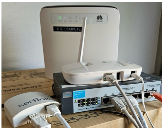
Figure 10 Test of two different Kerlink LoRaWAN gateways (Kerlink Wirnet iZeptoCell Ethernet 868 MHz on the left, Kerlink Wirnet iFemtoCell LoRaWAN Gateway 868 MHz on the right).
