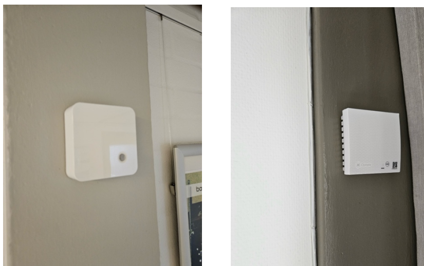
Figure 6 Left: Elsys ERS CO2 sensor. Right: MClimate CO2 Sensor & Notifier. While the MClimate sensor operates on standard AA 1.5 V batteries (with up to 10 years of battery life), the Elsys ERS CO2 sensor uses industrial 3.6 V AA batteries, offering a battery life of over 11 years with data reading and sending every 10 minutes. The Elsys CO2 sensor includes an incorporated PIR sensor and is slightly more costly than the MClimate sensor.
