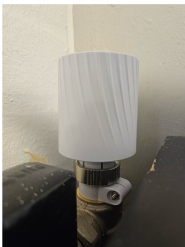
Figure 9 Left: MClimate Vicki thermostatic head. Center and right: Vicki plexiglass cover.
