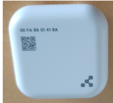
Figure 7 Bluetooth beacons are used to locate users of the FeedMe app within buildings, facilitating the feedback collection process. Users do not need to manually select which room they are in; the app automatically recognizes the room based on proximity to the room's beacon.
