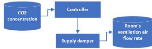
Fig. 4 – Room ventilation model
