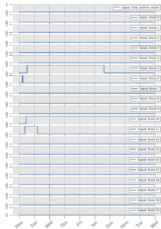
Fig. 12 – Anomaly signals for the rooms of the ventilation system
