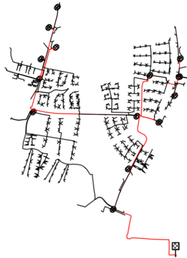
Figure 13: Case study of the Danish grid, showing 10 kV and 0.4 kV cables, along with transformers and the 60/10 kV connection. Red lines represent 10 kV cables, and black lines represent 0.4 kV cables. The grid supplies 822 consumers.
