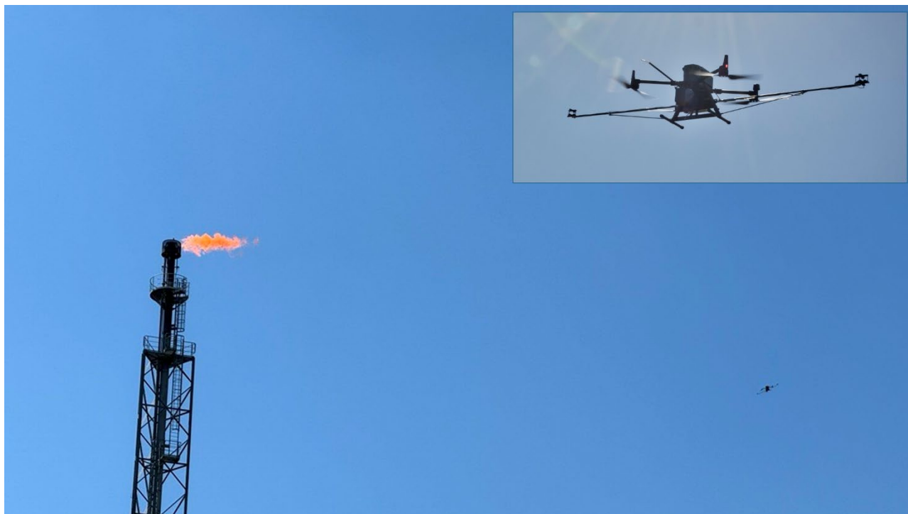
Figure 1: Example of a drone-borne measurement for the calculation of DRE in the in-situ environment. The photograph in the upper-right corner shows the drone setup with sensors in greater detail.
