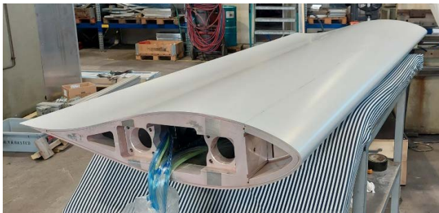
Figure 13: Left: The FFA-W3-211 after coating. Right: example of an IR picture where transition is visible ( Re=3E6 , AoA=8.5 deg., pressure side, LER-2).
