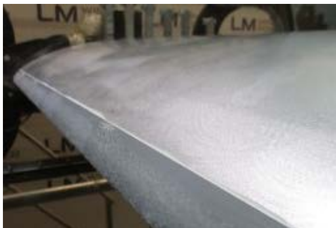
Figure 15: LE1 mounted on the DU00-W-212 in LM's wind tunnel.
