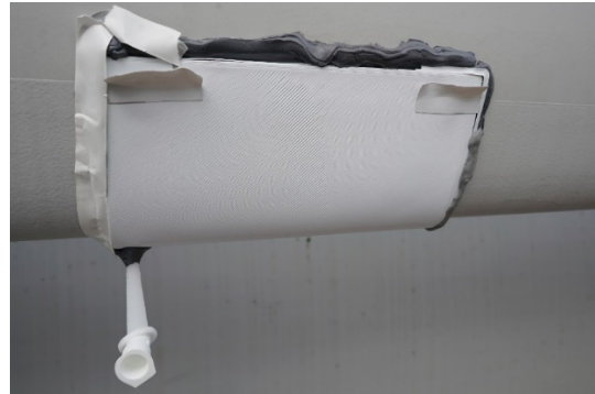
2: Mould for silicone imprint on the blade
