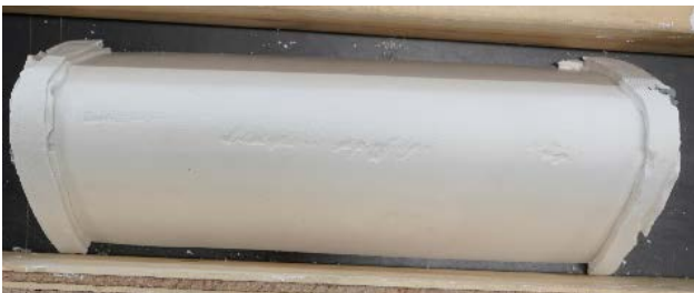
1: Wind turbine blade with LER
