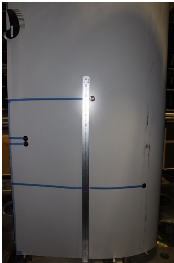
Figure 21: Locations of the surface microphones on the suction side of the FFA-W3-211 aerofoil.
