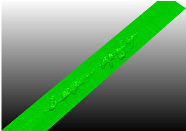
3: Plaster casting of the LER
