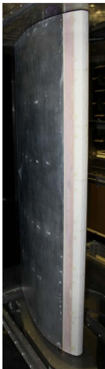
Figure 14: LER-2 mounted on the DU91-W2-250 in PLCT.
