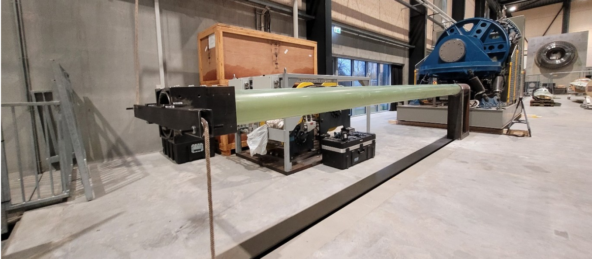
Figure 45: Test setup for applying pure torsion.
