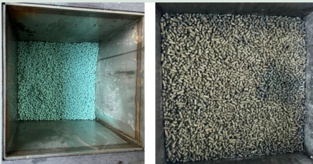
FIGURE 32. Left: Fresh sulphur guard installed November 17 th at Ejby Mølle. Right: Spent sulphur guard removed after pilot dismantling in Tårnby.
