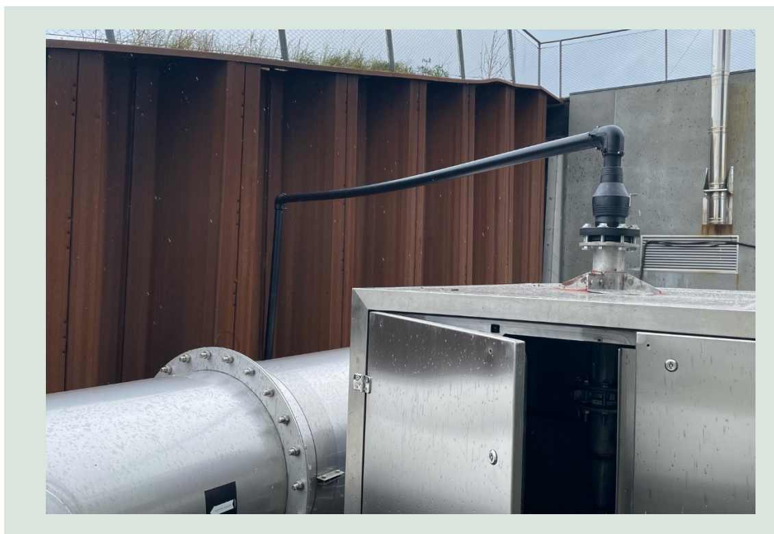
FIGURE 5. Pipe connection from the process tanks off-gas to the pilot plant in HCR Syd before heat tracing and insulation.
