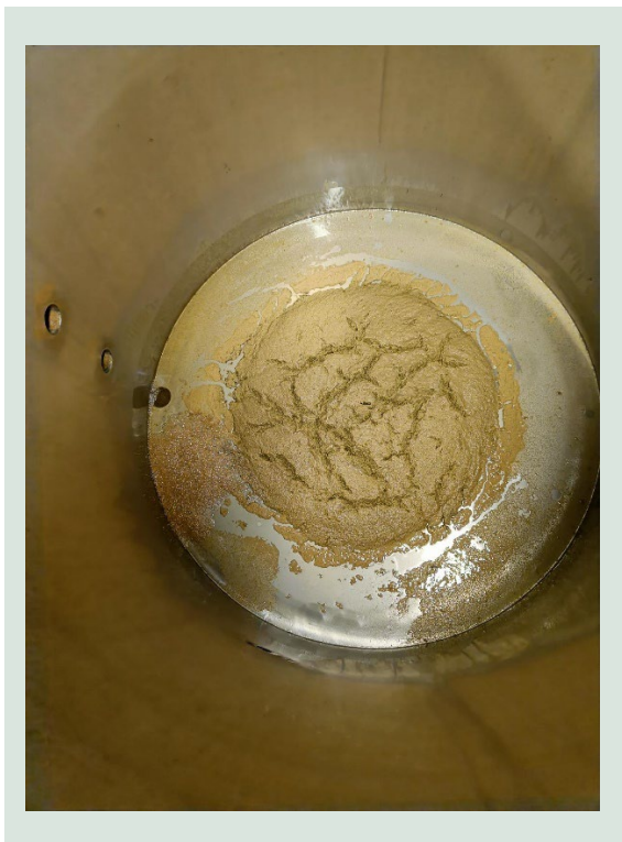
FIGURE 4.13. Deposited trub when experimenting with Brew 15 without carbonation – 30 min boiling.
