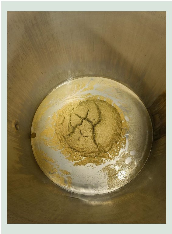
FIGURE 4.122. Deposited tube when experimenting with Brew 14 with carbonation – 30 min boiling.
