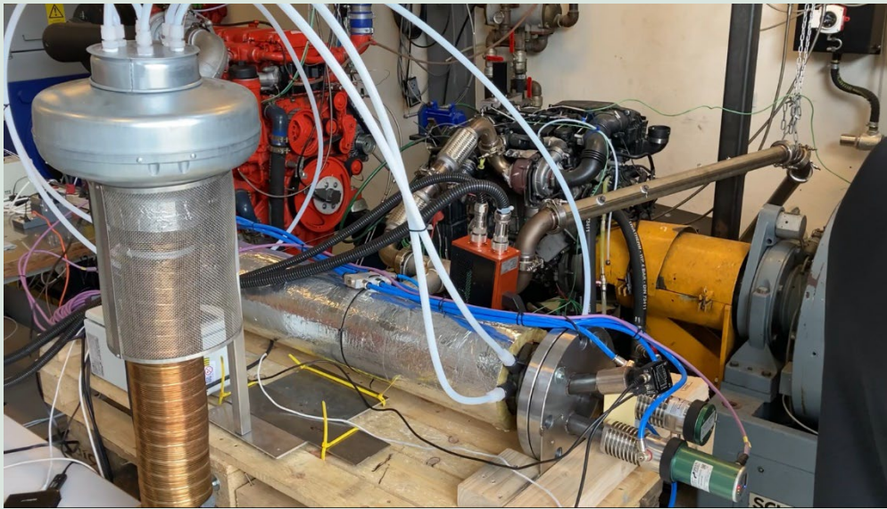
FIGURE 5. Diesel engine set-up with EMS BC sensor installed in the extractive tube.
