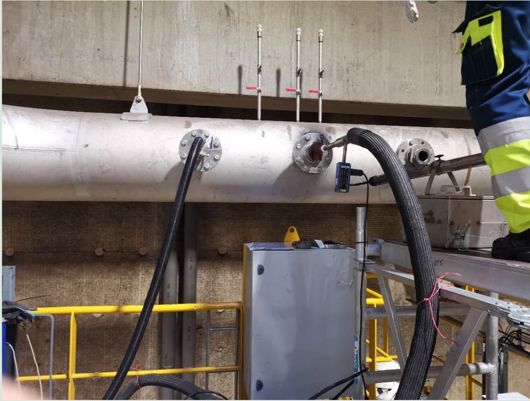
FIGURE 4. Gas Measurement Connections From left to right, the following measurements were taken: Black carbon (BC), ELPI (Electrical Low-Pressure Impactor), and particle matter (PM).
