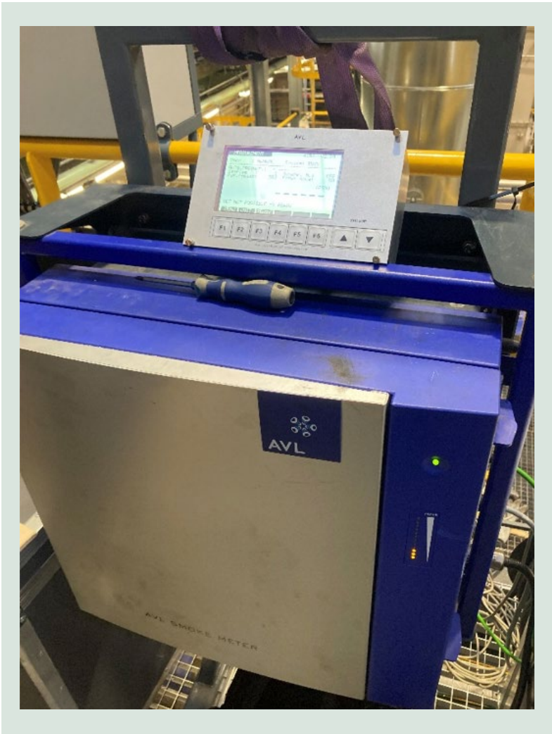
FIGURE 5. AVL Smoke Meter applied for measuring before and after the ESP.
