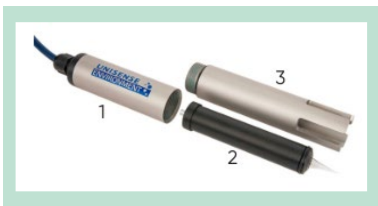
FIGURE 18. The three components of the Unisense Environment A/S N_2O wastewater sensor, showing: (1) the sensor body, (2) the sensor head and (3) the sensor protection tube. The sensor body also contains a temperature sensor. (Unisense Environment A/S, 2023).
