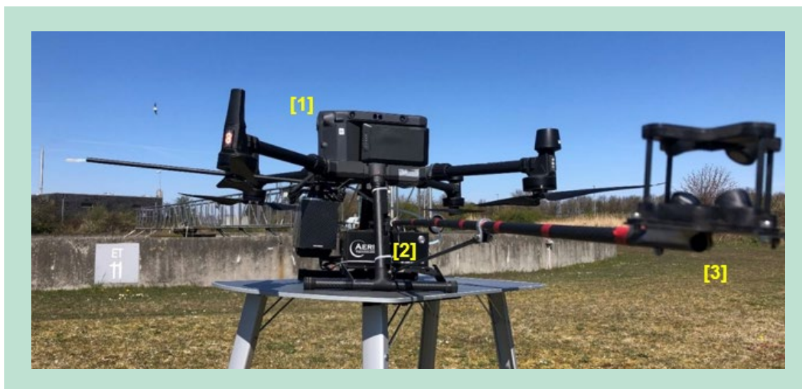
FIGURE 2. UAV (1) equipped with the Aeris Mira Strato N 2 O (2) and Aeris wind sensor (3).
