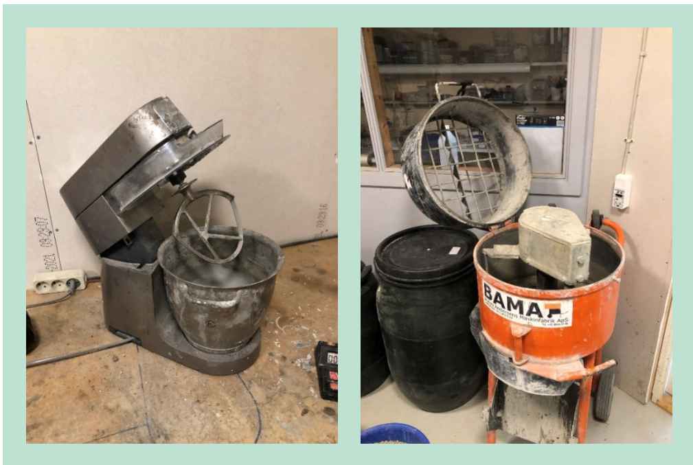
FIGURE 1. Kenwood benchtop kitchen mixing unit capable of mixing 2-3 kg concrete batches (left) and BAMA planetary mixer capable of mixing 30 kg concrete batches (Right).
