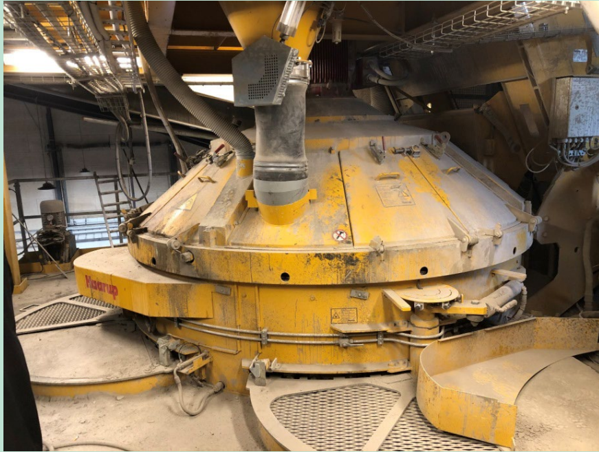
FIGURE 2. IBF's Industrial mixing unit capable of mixing 2.5 ton concrete batches.
