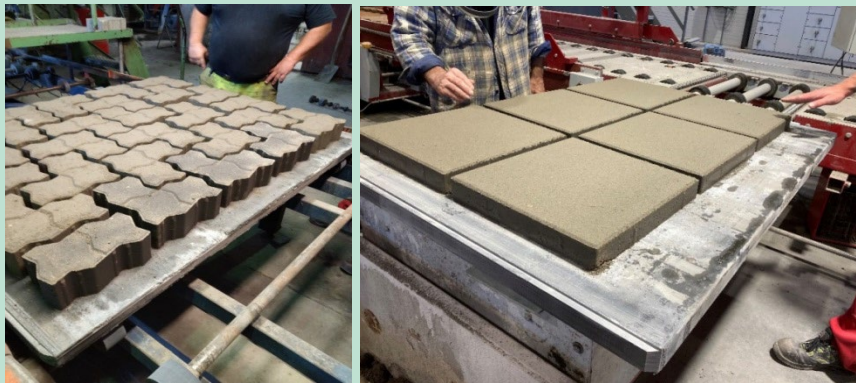
FIGURE 3. Green state, Coloc blocks (left) and Paving stones (right), directly after ejection from IBF's vibration compression unit.
