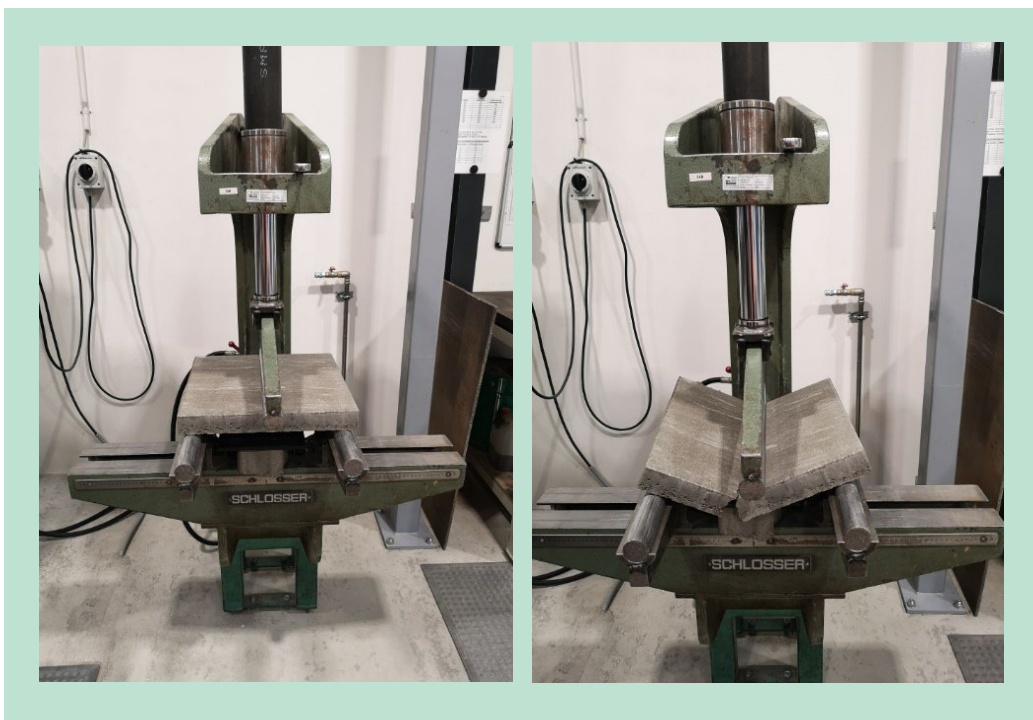
FIGURE 11. Hydraulic mechanical test equipment used to measure bending strength.
