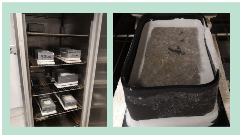
FIGURE 12. Left, specimens in freezer and right an example of a specimen with rubber sheet and salted water covering sides and top respectively.
