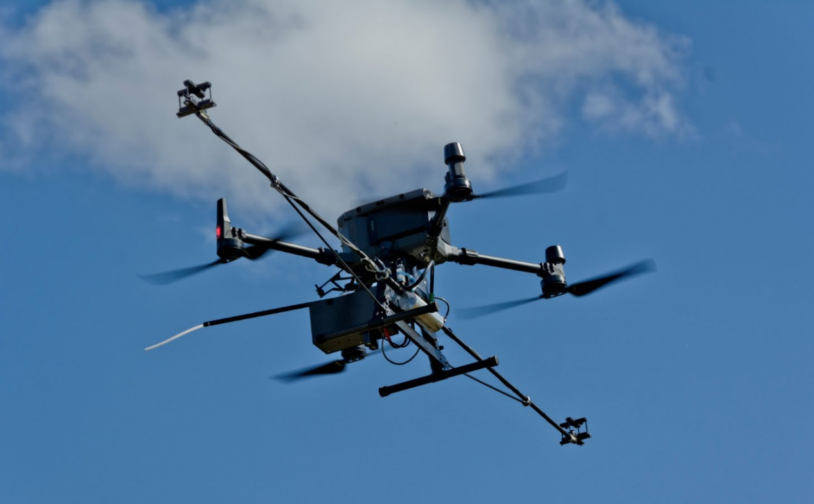
Explicit's drone equipped with a methane gas sensor and two wind sensors.
