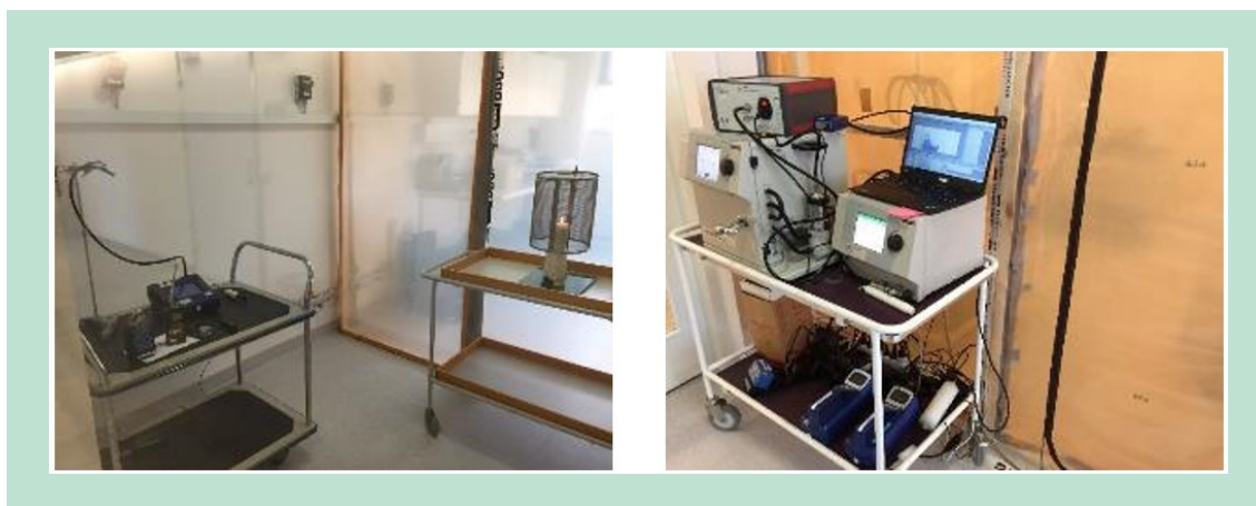
FIGURE 2. LEFT: Sampling position 2 with DustTrak and pumps for filter collection on the roller table to the left. A burning candle can be seen on the roller table to the right. RIGHT: Roller table with SMPS equipment outside the climate chamber.
