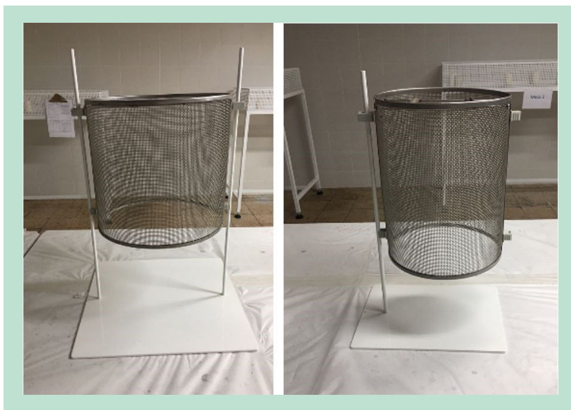
FIGURE 1. Example of sooting test equipment (diverse diameters for different diameter candles).
