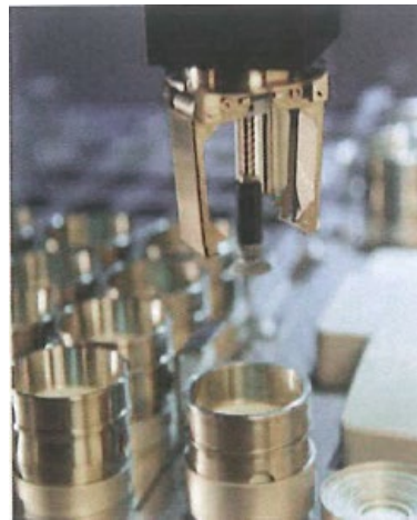
Figur 1.1 Sample changer picking up a sample in the priority position
