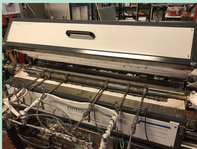
FIGURE 7 The bench-scale setup for small monolith samples at the Technical University of Denmark.
