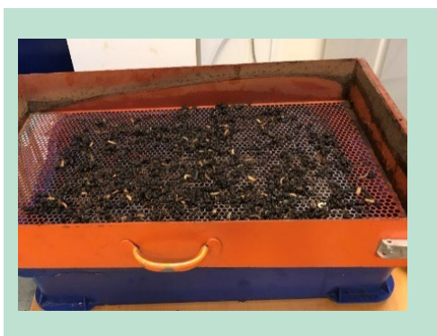
FIGURE 33. Separation of BSFL and insect frass using a migratory approach.
