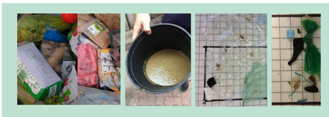
FIGURE 2. Processing from former foodstuffs to bio-pulp. From left: Former foodstuffs delivered to Daka ReFood; Final bio-pulp; Examples of impurities detected from final bio-pulp.
