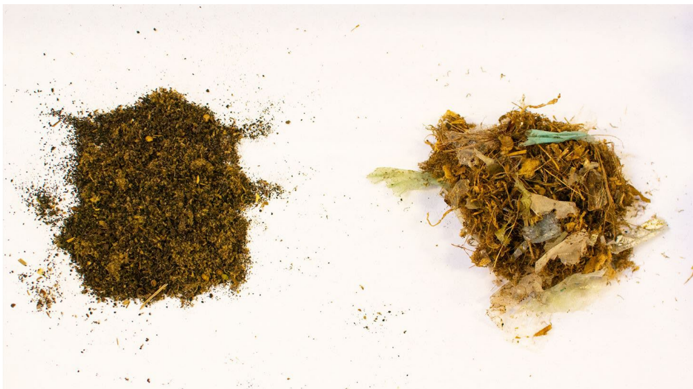
Picture: Technical frass (left) separated from impurities original in bio-pulp
