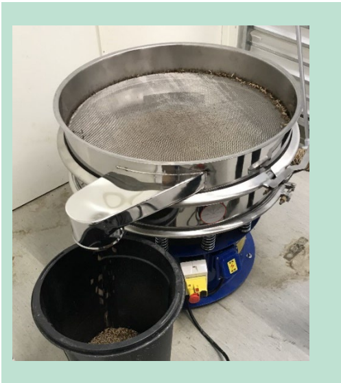
FIGURE 35. Separation of BSFL and insect frass using mechanical sieving.
