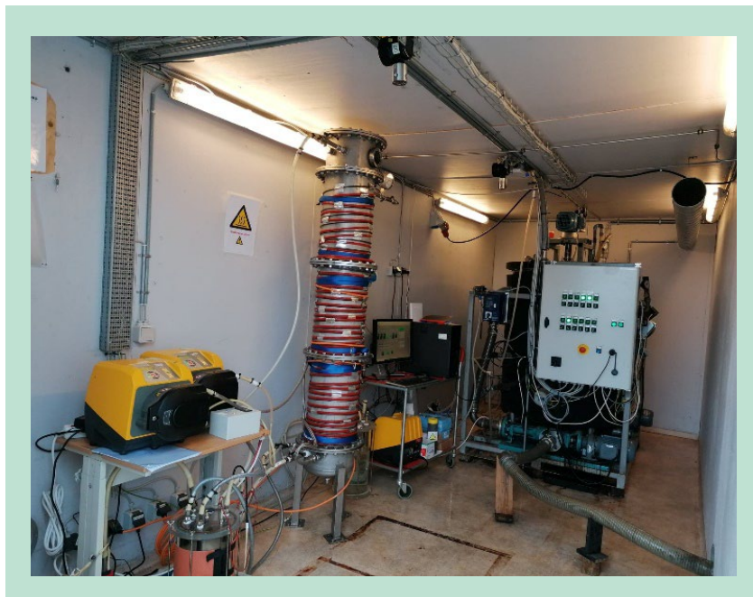
FIGURE 6. Pilot-scale operation at BIOFOS WWTP in Avedøre. Left: biological upgrading TBR. Right: Anaerobic digestion reactor.
