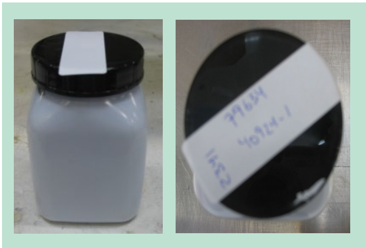
FIGURE 1. Reference samples from each produced batch of paint are collected in 250 mL plastic jars.
