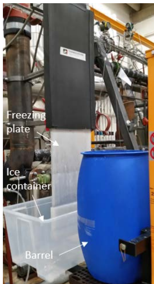
Figure 11. Test setup for freeze concentration
