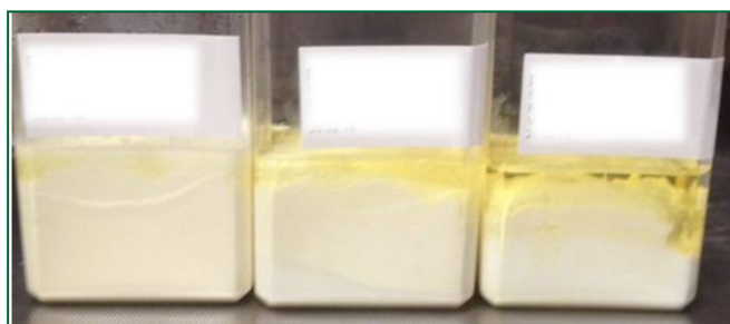
Figure 6 An example of emulsion instability. The three containers have the same oil-in-water (O/W) formulation (a sun spray) at three different pH levels; pH from left to right: 5.9, 5 and 4.5. A phase separation clearly occurs when pH is decreased, and at pH 4.5 the separation of the oil phase (top) from the water phase (bottom) is clearly visible.
