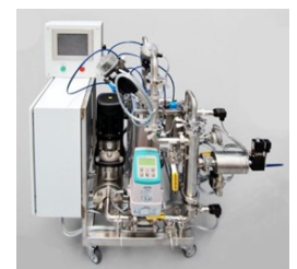
LiqTech LabBrain Pilot unit used for testing prototype in Denmark
