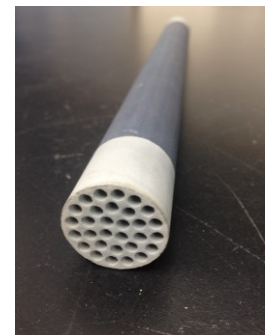
Prototype The membrane prototype has an outer diameter of 25 mm, length of 305 mm, and 30 channels, each of 3 mm diameter
