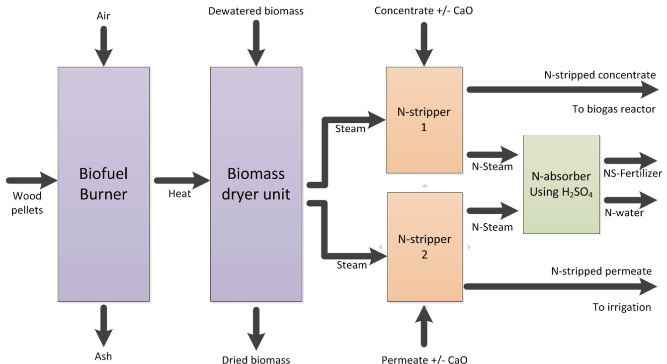
Figure 3. Simplified overview of the biomass dryer unit and the nitrogen stripper units of the New Substrate Concept.
