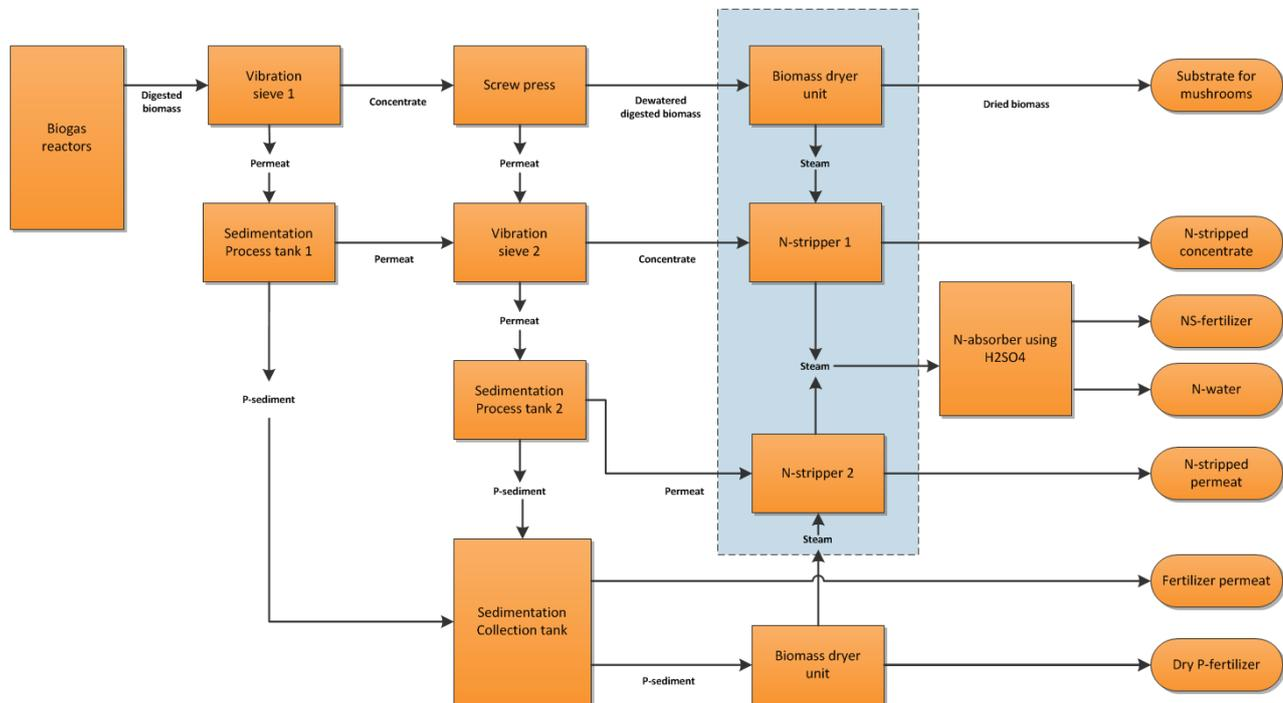
Figure 2. Overview of the different components in the complete New Substrate Technology Concept. Note that in most cases only one biomass dryer unit will be included since one dryer unit normally will have sufficient capacity to treat both the dewatered digested biomass and the P-sediment. The present verification focusses on the key components highlighted in the blue box: 1) The biomass dryer unit (drum dryer) including a biofuel burner unit. 2) The two N-stripper units.
