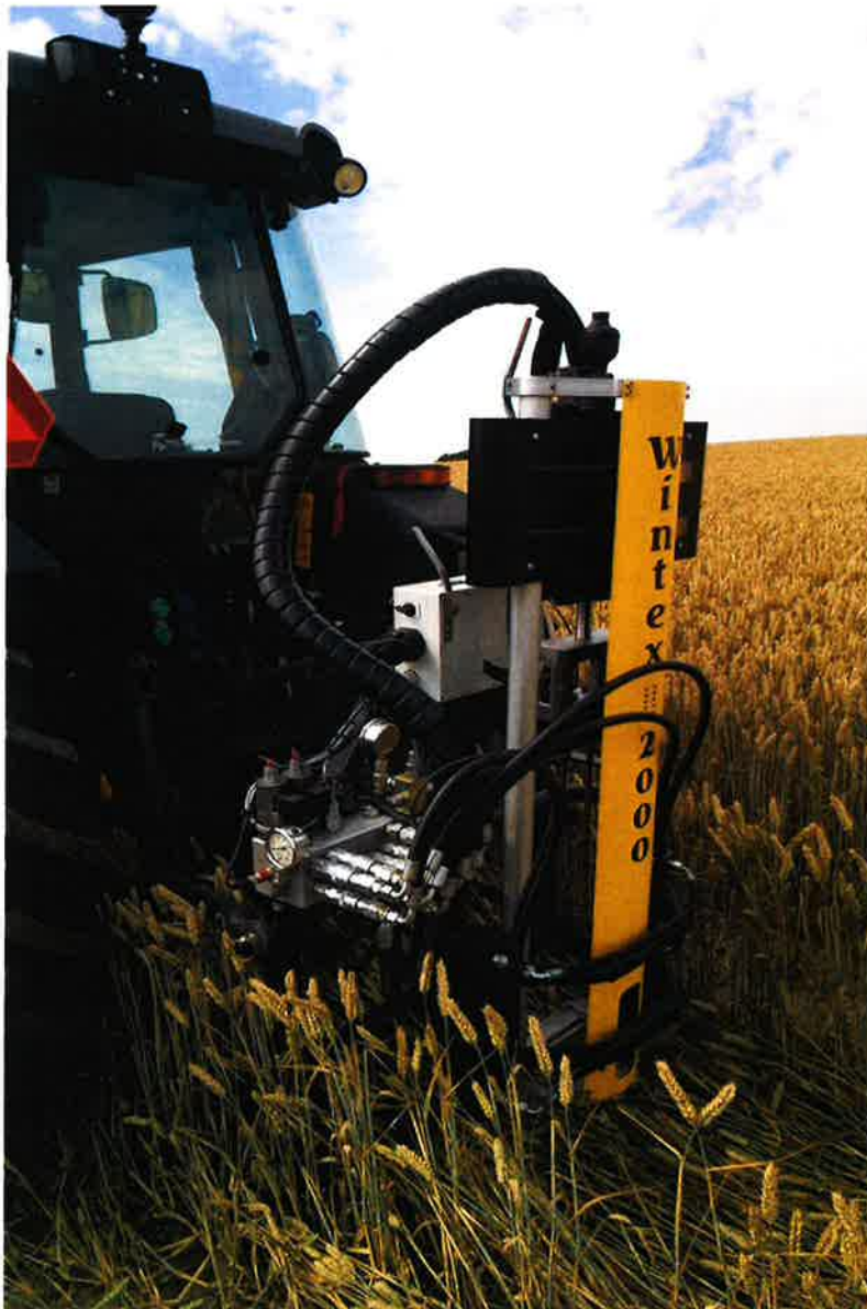
Figure 1. The Wintex 2000 configured for soil moisture measurement and mounted on a standard farm tractor
