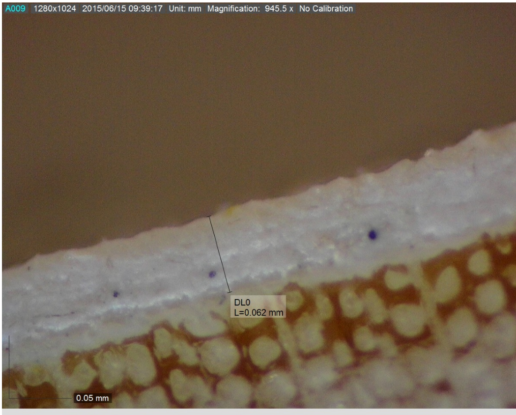
IMAGE 10 CROSS-SECTION MICROSCOPY IMAGE OF A CROSS-SECTION OF THE REFERENCE SYSTEM 923.
