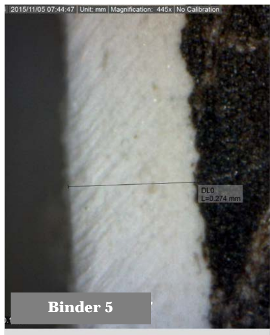
IMAGE 11 CROSS-SECTION MICROSCOPY IMAGE OF A THE INDUSTRIAL PRIMER SAMPLES AFTER THE TANNIN-BLOCKING TESTS. BINDER 2 IS INCLUDED AS AN ALTERNATIVE REFERENCE FOR A PRIMER SYSTEM.
