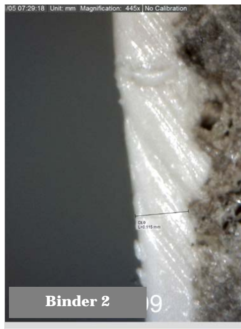
IMAGE 11 CROSS-SECTION MICROSCOPY IMAGE OF A THE INDUSTRIAL PRIMER SAMPLES AFTER THE TANNIN-BLOCKING TESTS. BINDER 2 IS INCLUDED AS AN ALTERNATIVE REFERENCE FOR A PRIMER SYSTEM.
