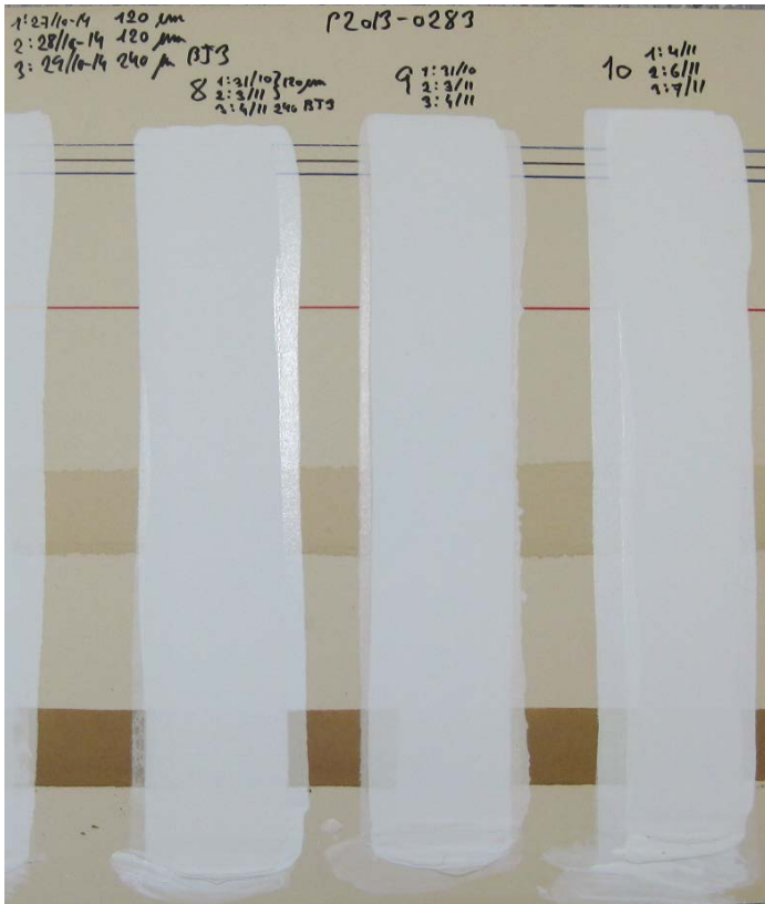
IMAGE 5 STAIN-BLOCKING TESTS WITH SELECTED BINDERS FOR THE SEALING PRIMER. HORIZONTAL LINES ARE (STARTING FROM THE TOP): THREE DIFFERENT BALL PENS, A PERMANENT MARKER, NICOTINE AND COFFEE. VERTICAL WHITE LINES ARE PRIMERS WITH DIFFERENT BINDERS (STARTING FROM LEFT): REF. NO. 8, 9 AND 10 (SEE TABLE 3 OR TABLE 8 FOR REFERENCE NUMBERS).
