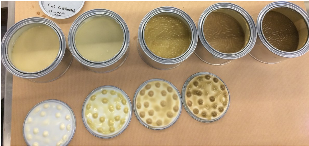
IMAGE 15 PHOTOGRAPHS OF CORE-SHELL ENCAPSULATED SICCATIVES IN WOOD-PROTECTING PAINTS. UNDESIRABLE DRYING EVENTS ARE OBSERVED FOR HIGHER LOAD LEVELS OF SICCATIVE (SAMPLES TO THE RIGHT). THE CHANGE IN COLOR IS SPECULATED TO RESULT FROM OXIDATION OF THE COBALT SICCATIVE.
