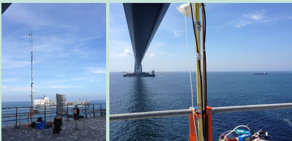
FIGURE 8 MEASUREMENT POSITION 6 M ABOVE THE PYLON PLATFORM AS WELL AS 2 M ABOVE THE PLATFORM (PICTURES FROM CAMPAIGN IN JUNE 2014).
