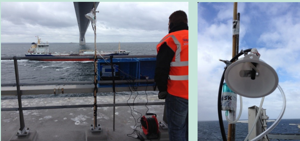
FIGURE 6 VIEW FROM THE MEASUREMENT POSITION AT THE EASTERN PYLON PLATFORM OF THE GREAT BELT BRIDGE (LEFT) WITH A NORTHBOUND SHIP SHOWN. THE GAS INTAKE TO THE SENSORS IS SHOWN TO THE RIGHT.
