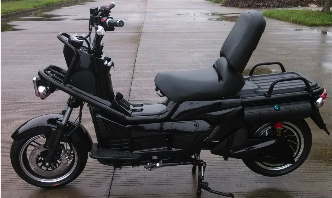
BILLEDE 9 IEV CARGO , 4KW BRUSHLESS IN-WHEEL MOTOR, 60V/100AH LI-ION BATTERI
