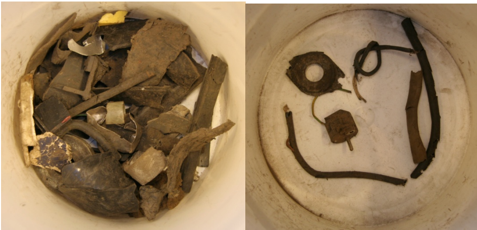
Figure 4.7 SR items sorted with PGNAA sensor. Left: chlorine-free items; Right: chlorine-containing items (Force Technology).
