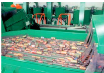
Figure 3.10 X-Ray sensor sorter at the UNI-CYC plant in Bremerhaven 53
