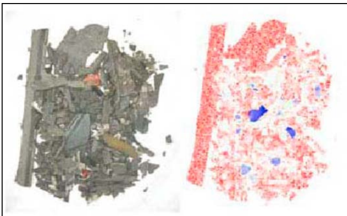
Figure 3.5 Normal picture (left) and XRT image (right) of hand sorted plastic fraction. The XRT image reveals flame retardant plastics (dark blue) and PVC (pink). (Delft University of Technology)
