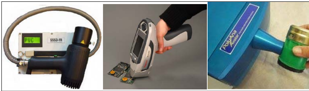
Figure 3.1 SSS3-FR - Sliding Spark Spectrometer for Fire Retardants detection 47 , Niton XFR from Thermo Scientific 48 , PolyAna from Wolfson Electrostatics 49
