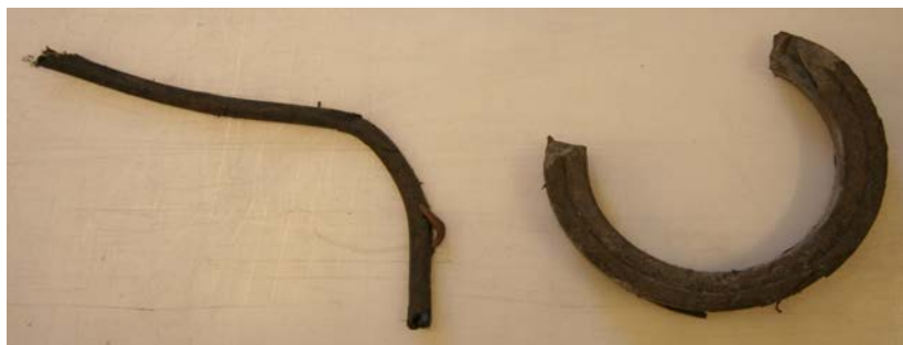
Figure 4.5 SR items used for demonstration of the sensitivity of the PGNAA sensor. Left: chlorine-containing material (16.8 g); Right: chlorine-free material (123 g)
