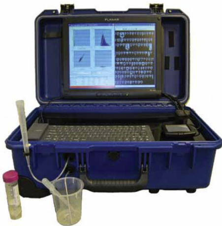
Figure 21. BallastCam © from Fluid Imaging Technologies, developed to conduct indicative sampling and analysis onboard the ship.
